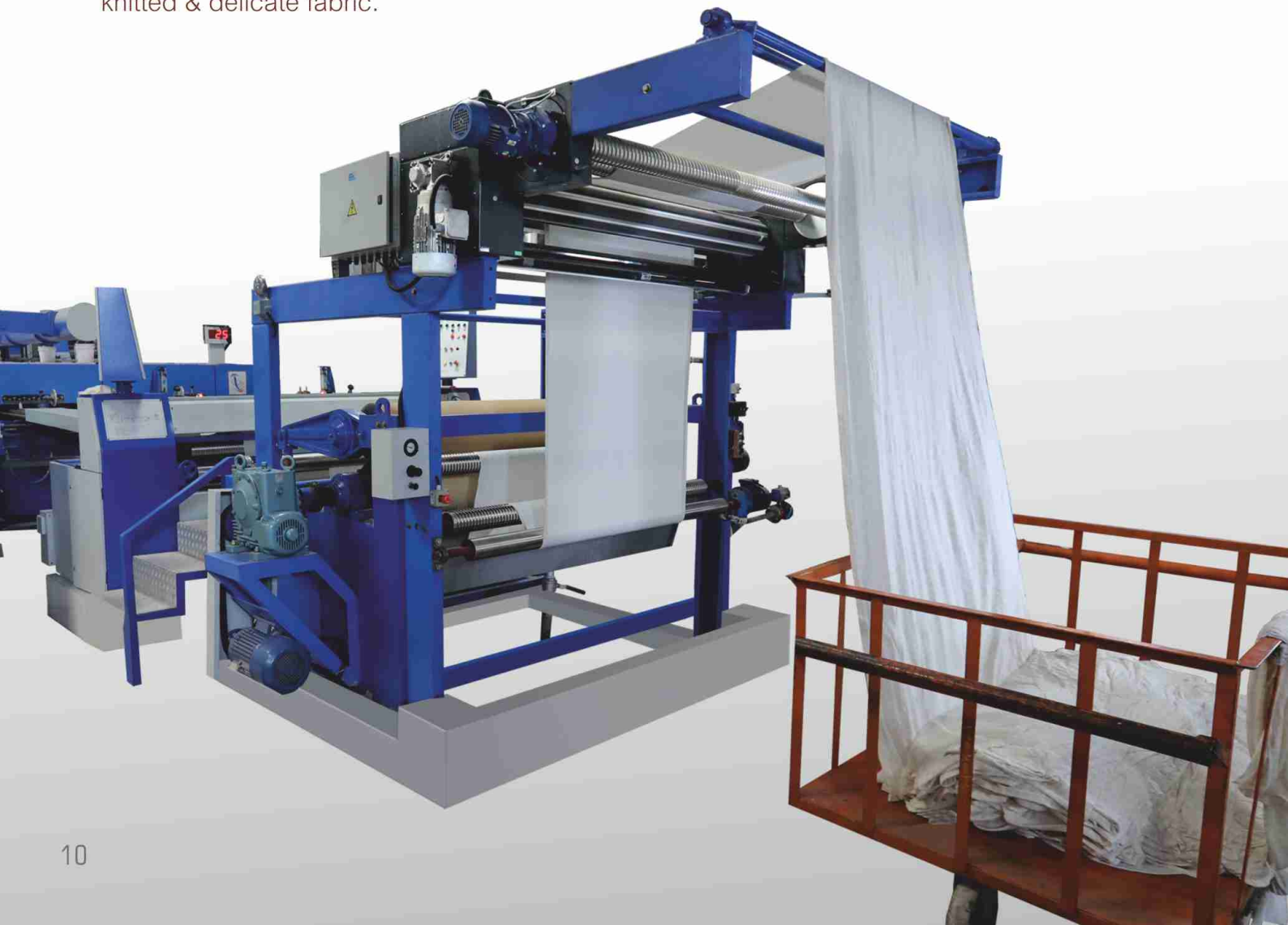
Inlet arrangement with centering device suitable for knitted & delicate fabric.
